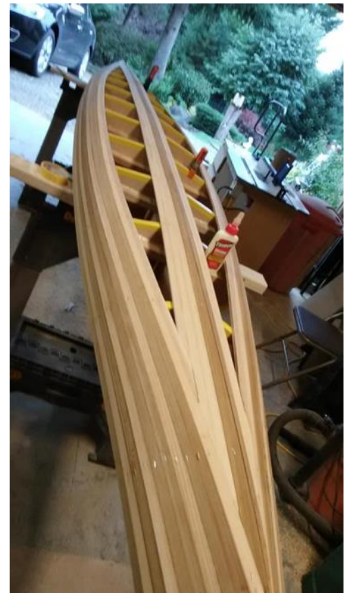
Wood strips being laid on the hull ribs.
